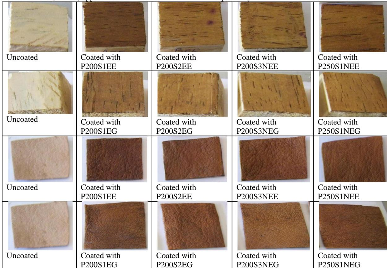
**Plate 2:** Uncoated and Coated Wood and Leather respectively
