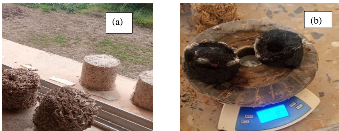
Figure 4: Briquettes used for fuel for consumption rate test (a) before and (b) after combustion
