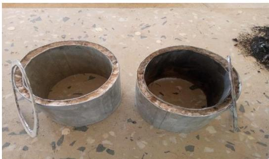
**Figure 1:** fiber glass combustion chamber
