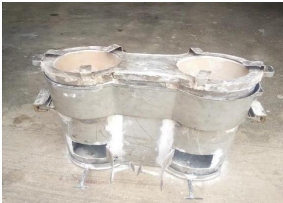
Figure 4: Pictorial view of the developed cookstove
